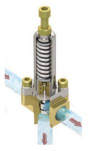
for 900 PSI operation, the PRV simply bypasses 2 GPM and the pressure remains steady at 900 PSI. So as long as you size your pump properly and want to use the same pressure range for all the tools, this approach is very simple and requires no adjustments to the motor speed or setting of the PRV.
